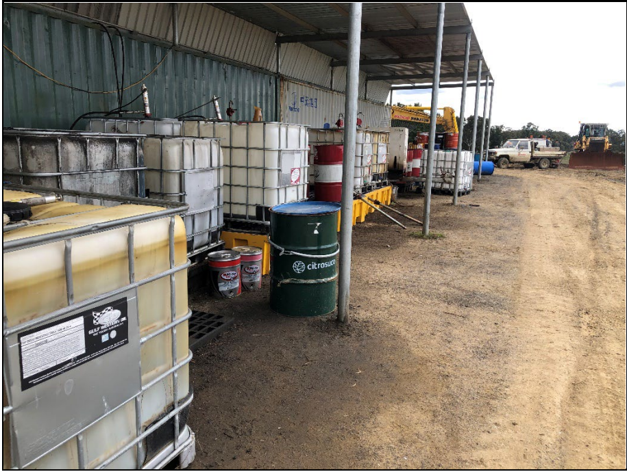
Photo 15: Lubricant storage at maintenance workshop. Most items stored on portable bunds. Some soil staining evident.
