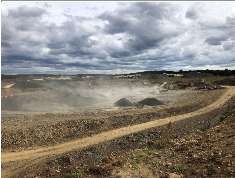
Photo 10: Basalt Extraction area looking north west showing dust generated by basalt processing equipment.
